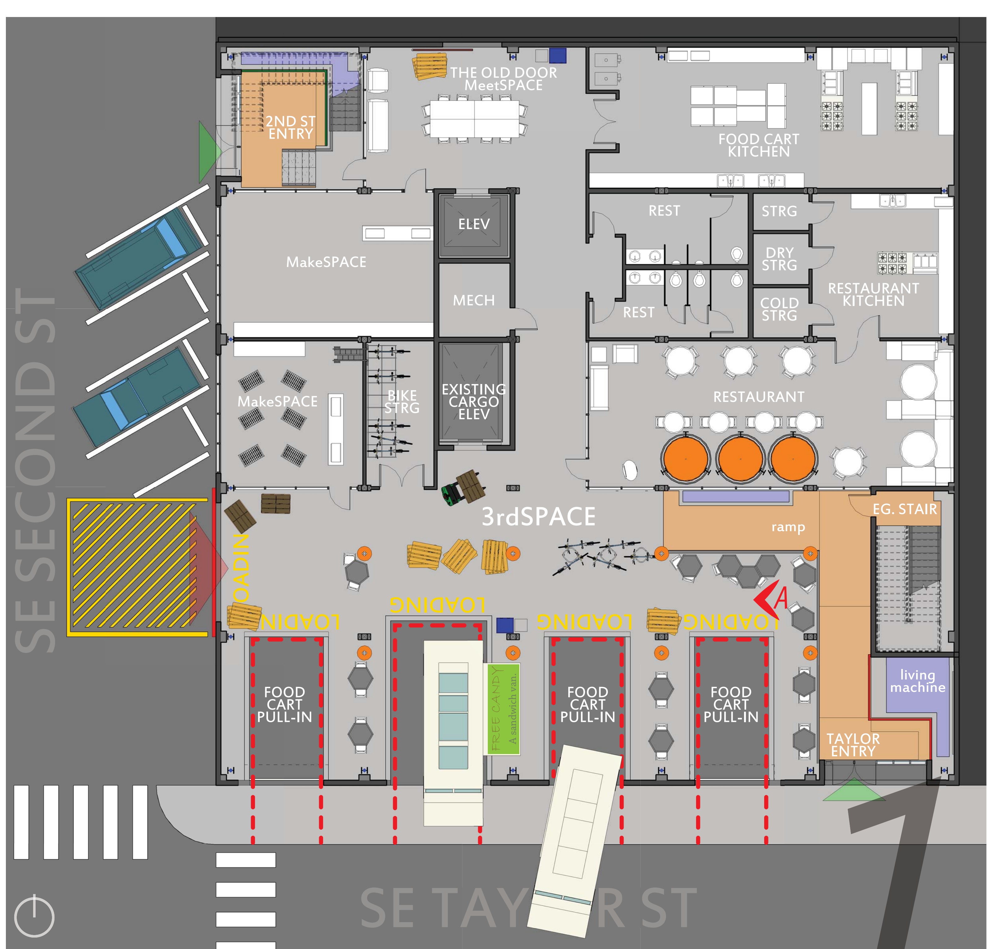
Ground Floor Plan - 1/8" | Challenges - New interior wall partitions within the existing timber grid structure. - New stair and elevator cores added for seismic strength and upper floor support. - New entry ADA access.
