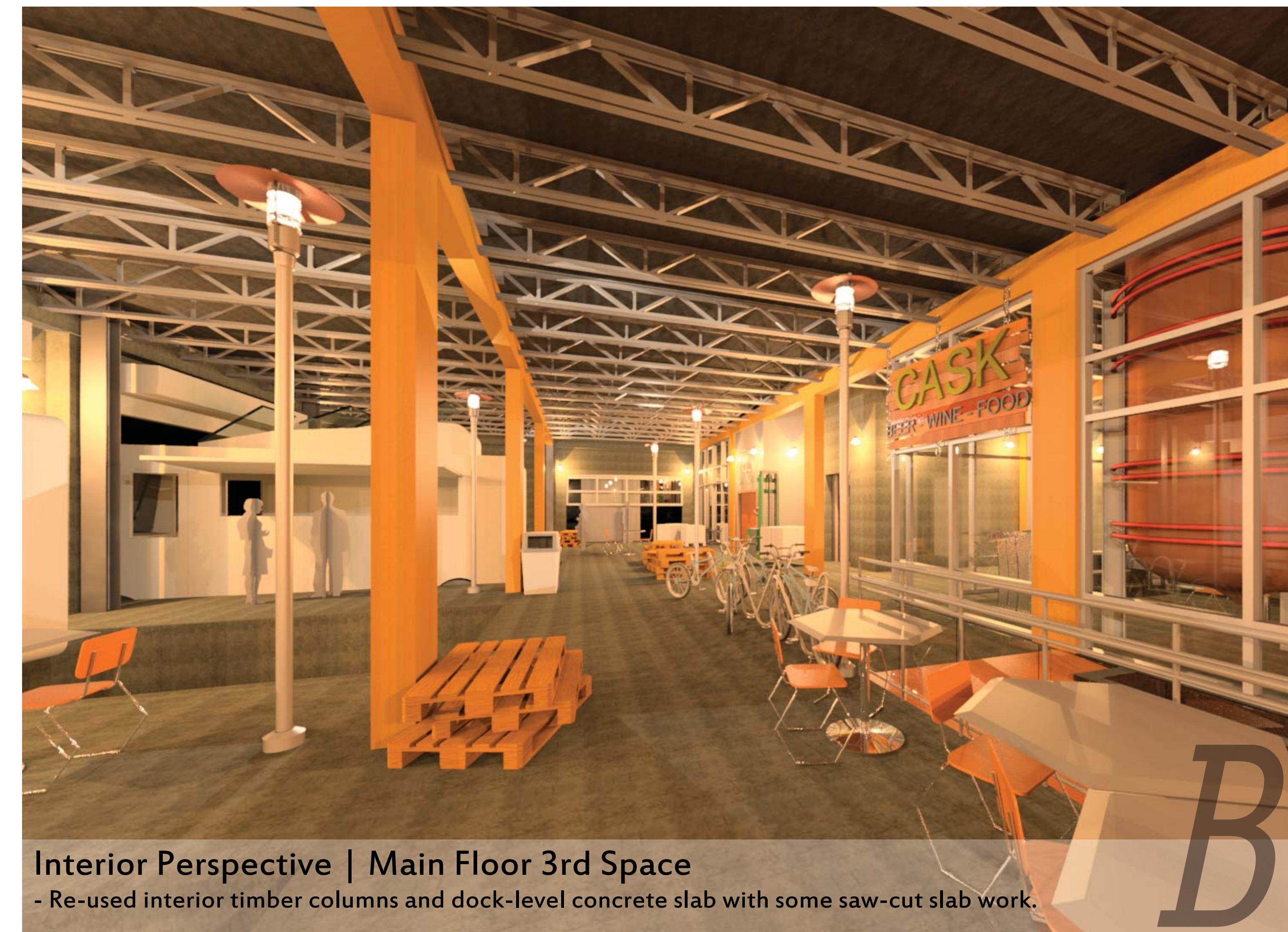
Interior Perspective | Main Floor 3rd Space - Re-used interior timber columns and dock-level concrete slab with some saw-cut slab work.
